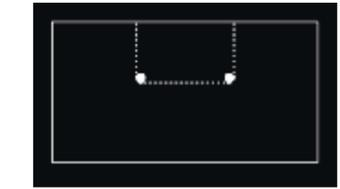
When cutting a “U” shaped piece, Mark and drill relief holes where the cut lines intersect, always making the shortest cut first.
