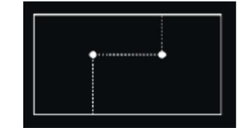
When cutting an “L” counter top, drill relief holes where the cut lines intersect, always making the shortest cut first
