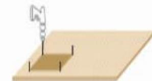
Use a drill bit 3 to 5 mm to drill corners of the cut-out.
